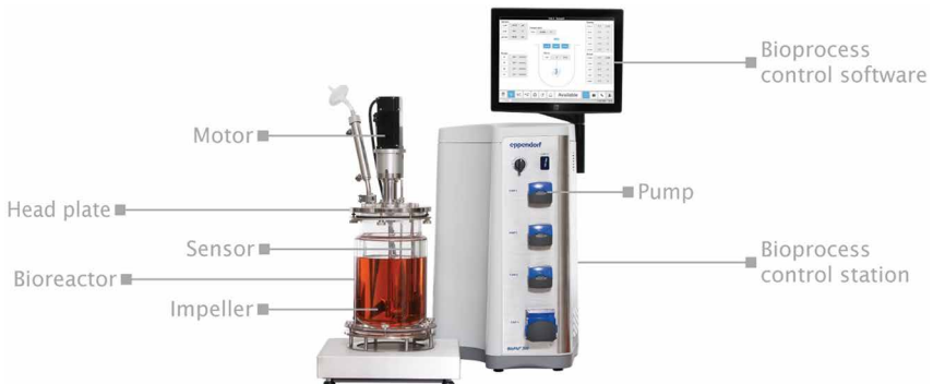
Figure 1 Profile of a bioreactor. Components of a stirred tank-bioreactor (left) and a connected control station (right).
