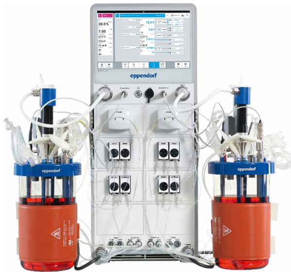
Figure 5 Two bioreactors wrapped in heating jackets and attached to a bioprocess control station. Besides electrical heating jackets, water jackets can be an option for temperature control in a bioreactor. The optimal growth temperature is regulated and maintained by the control station.
